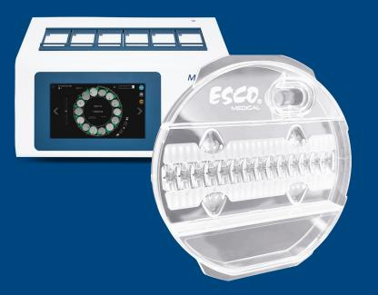
The lid is mounted inside the circumference of the dish covering the culture area completely – the user will only grab the dish during handling and not risk losing the dish by holding on to the lid only – as can be the case on all traditionally designed dishes. A large well is provided outside the culture area for pH measuring without affecting the cultured samples. The dish has a flat bottom so it is ideal for heat transfer from below.
