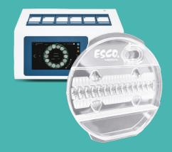
The lid is mounted inside the circumference of the dish covering the culture area completely – the user will only grab the dish during handling and not risk losing the dish by holding on to the lid only – as can be the case on all traditionally designed dishes. A large well is provided outside the culture area for pH measuring without affecting the cultured samples. The dish has a flat bottom so it is ideal for heat transfer from below.
