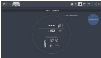
The user can plug any standard BNC pH probe into the unit and measure the pH in the samples at will.
