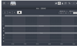
Conditions that put the MIRI® into alarm state are recorded. It is possible for the software to send email alerts as well
